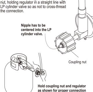
**6.**Turn the coupling nut clockwise and tighten to a full stop. The regulator will seal on the back-check feature in the LP cylinder valve, resulting in some resistance. **An additional one-half to three-quarters turn is required to complete the connection. Tighten by hand only – do not use tools.**
